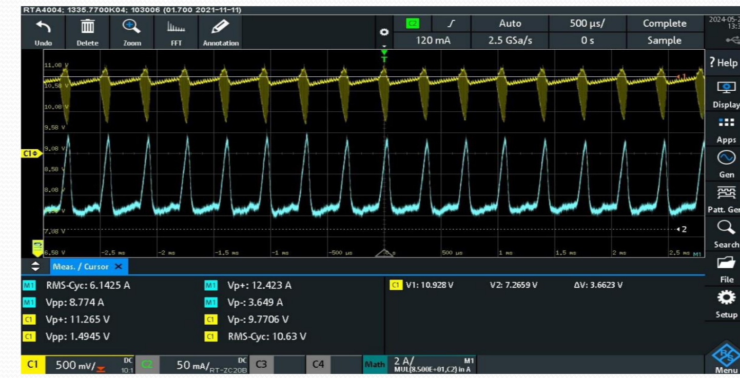
Voltage and current graph under full-load condition
