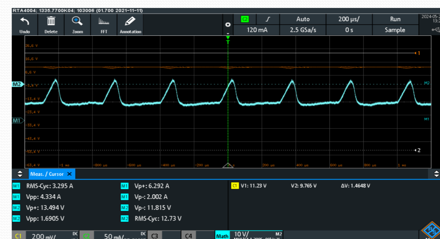
Voltage and current graph under half-load condition
